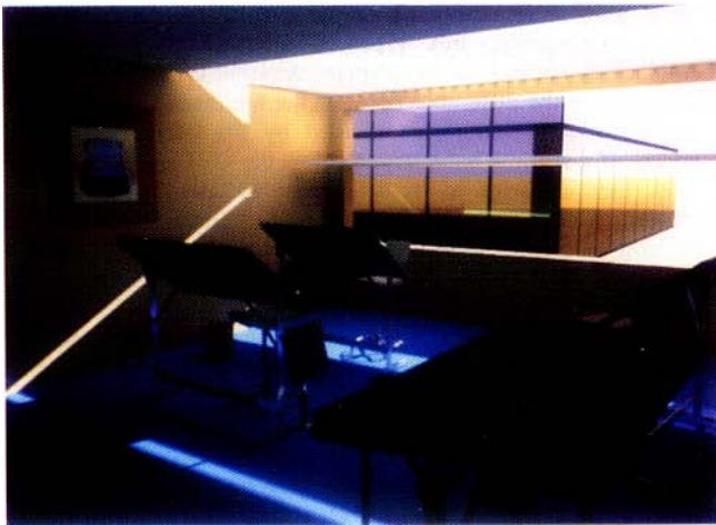
Figure 9a. A drafting office with a mirror light shelf slicing the window and redirecting light upwards.
