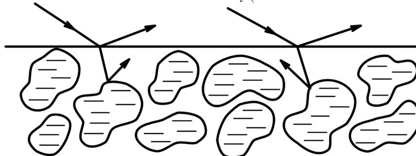
Figure 2 : Surface and subsurface reflection on a plastic material
