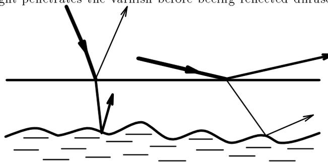
Figure 3 : Influence of the incident angle on surface and subsurface reflection
